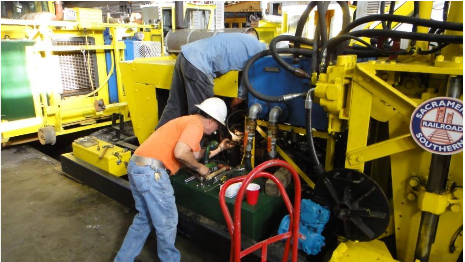
Mike H. and Fred work on removing the old malfunctioning air compressor on the tie-shear.
