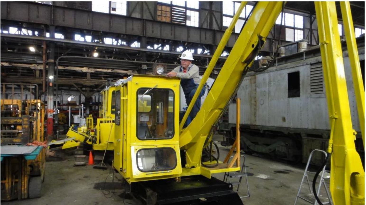
Cliff fits new shields on the headlight of the tie-crane, which is looking quite yellow thanks to Alan's artistry...
